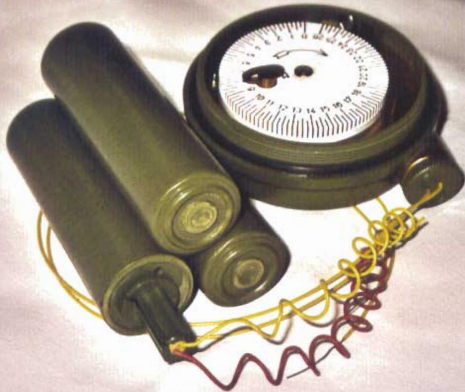
Time delayed explosive device with mechanical clock and TNT
