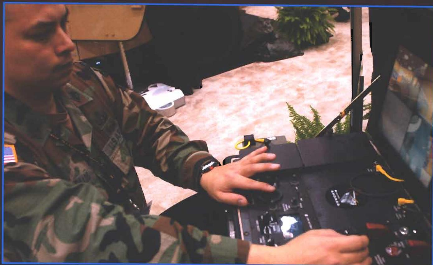
Staff Sgt. Santiago Tordillos operates the armed robotic system by remote control with two joy sticks on a control panel, tracking where it's going on a small screen. (Photo Courtesy of U.S. Army)
